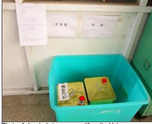
Photo of chemical storage room (if applicable) Chemicals were stored with secondary containment.JPG
