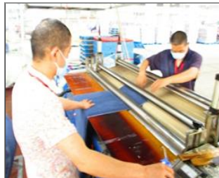
Photo of non-conformity The factory only provided worn dust proof masks instead of anti-poison respirators to gum worker.JPG
